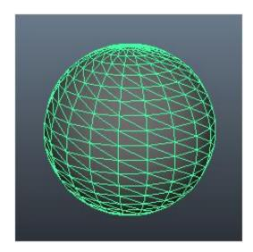
Each of the triangles in the sphere model has three points to it, we call each point a vertex. So for us to render the sphere model we need to put all the vertices that form the sphere into a special data array that we call a vertex buffer. Once all the points of the sphere model are in the vertex buffer we can then send the vertex buffer to the GPU so that it can render the model.
